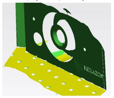
The display of the RT mesh has also been improved in this version. While measuring, the leading data is displayed as a point cloud for visualization until the mesh is computed and replaces this data set.
