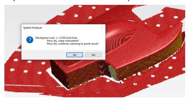
If a move has occurred a notification window will be displayed that includes an option to jump instrument and separate the data measured following the move.
